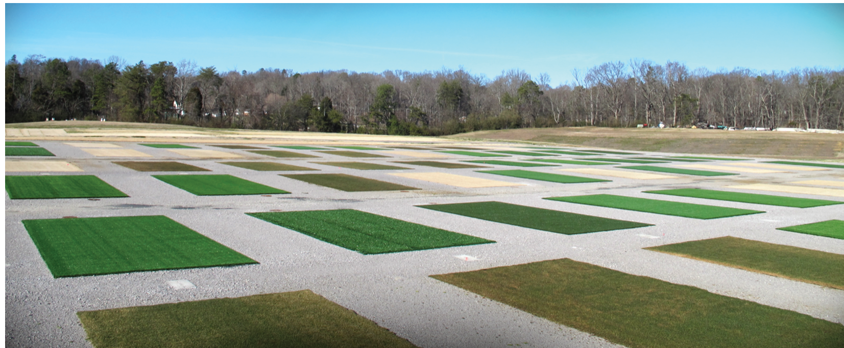
"The Farm" research center for the University of Tennessee - TurfGrass Science Department - Test plots of both natural and artificial turf allow the researchers to study the effects of weather and simulated game play in a large-scale, realistic environment.
